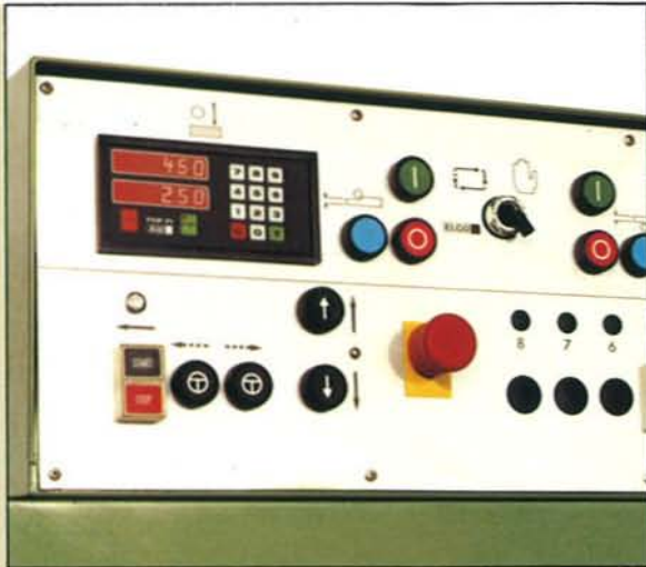
△ Electronic 'Dial-a-Size' giving quick and accurate positioning to the top and nearside heads, when small batches of a large variety of sizes are required, including automatic hydraulic slide locks.
